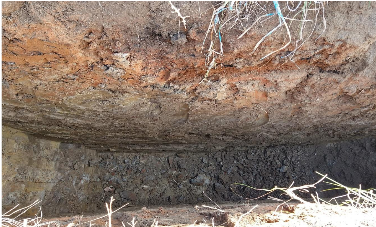
Photo 7: Test Pit 117 profile (Refusal at 2.2m) Typical of central and southern parts of Stage 1
